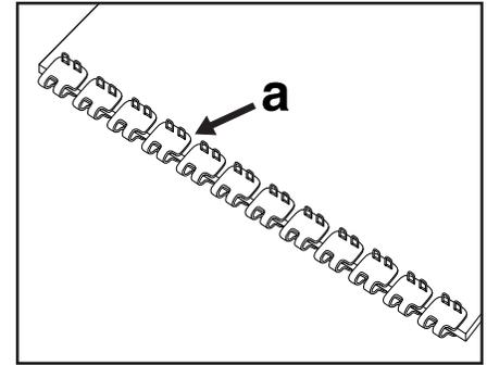
3. Place belt on solid surface for support. Center fastener strip, equal distance from the belt ends. (a) Staples should be facing up.
