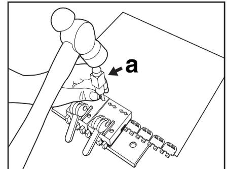
6. Starting with the center fastener plates, strike (a) staple driver with a 1 lb. (0.5 kg) hammer. Do not overdrive staples.
