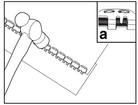
9. Set fastener strip flat on ST-28 setting plate. Strike top-side of fasteners and staples with firm hammer blows. Move back and forth across fastener strip until (a) staples clinch. Avoid hitting fastener loops. Repeat steps 1-9 on other belt end.
