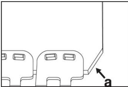
10. Using Belt Nippers, (a) notch trailing edge of belt only. Notch at an angle.
