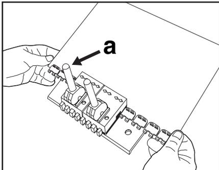
4. Center fastener strip in installation tool.
