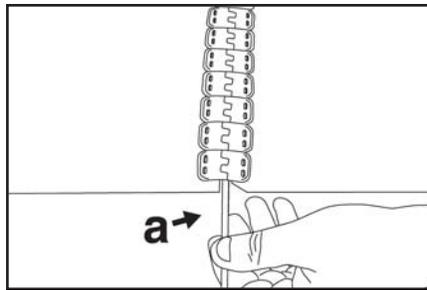
11. Bring belt ends together and (a) insert hinge pin. If retaining washer is used, crimp with pliers. Splice is complete.
